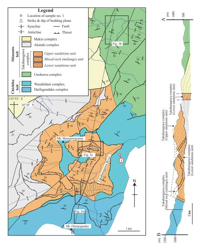
Fig. 2 Simplified geological map and cross section of the Yoshino area [modified from Takeuchi (1996) and Ota et al. (2019)].
