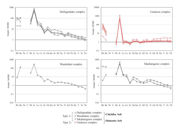
Fig. 8 MORB-normalized multi-element patterns of the examined samples. MORB composition normalization follows Sun and McDonough (1989).
