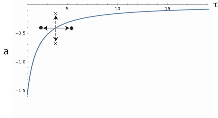
Figure 1: The stability boundary of the origin of Equation (1). The area with the curve and the axes is the stable region. Also, the schematics of the stochastic switchings are shown. Delay stochastic switching is between the two dot points indicated by the solid horizontal arrows, while the switching for the coefficients  $a$  is indicated by the two cross points with the dashed vertical arrows.
