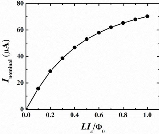
**Figure 3.** The nominal critical current dependence on the  $LI_c$  product normalized by  $\Phi_0$  for 0-0- $\pi$  SQUIDs according to the simulation. The critical current of 0-junction and  $K$  value are 50  $\mu\text{A}$  and 100, respectively.
