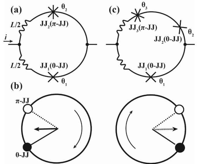
**Figure 1.** (a) Schematic of a  $0-\pi$  SQUID. (b) A pendulum model of the bi-stable states of a  $0-\pi$  SQUID. The white pendulums represent the  $\pi$ -junctions under upward gravity and the black pendulums represent the  $0$ -junctions under downward gravity. The solid and dotted arrows indicate that the phase of the  $0-\pi$  SQUID and total phase change between the bi-stable states is  $\pi$ . (c) Schematic of a  $0-0-\pi$  SQUID.
