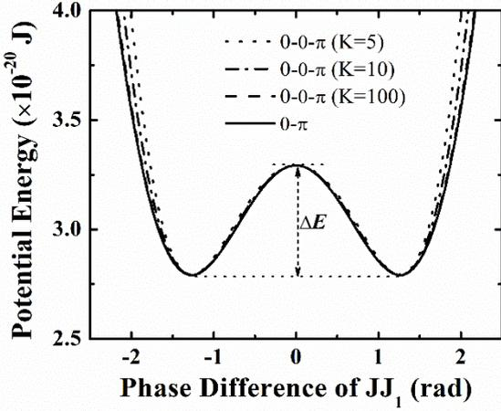
**Figure 2.** The potential energy of 0- $\pi$  and 0-0- $\pi$  SQUIDs as a function of the phase difference of  $JJ_1$ .  $K$  is the critical current ratio of the  $\pi$ -junctions to the 0-junctions of 0-0- $\pi$  SQUIDs with the same  $LI_c$  products ( $0.1\Phi_0$ )
