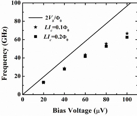
**Figure 5.** Maximum operating frequency as a function of bias voltage for different  $LI_c$  products in a JTL with LV-HSQ circuits. The solid line indicates the upper limit of  $f_{\max}$  (expressed as  $2V_b/\Phi_0$ ).
