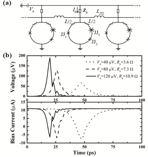
**Figure 4.** (a) Schematic of a JTL with HFQ circuit based on 0-0- $\pi$  SQUIDs, in which  $JJ_1$  and  $JJ_2$  are 0-junctions and  $JJ_3$  is a  $\pi$ -junction with  $K > 1$ . (b) The waveforms of voltages generated across the 10<sup>th</sup> 0-0- $\pi$  SQUID and bias currents flowing in the bias resistor  $R_b$  for different bias voltages  $V_b$ s.
