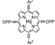
Fig. 1. Representation of magnesium diethynylporphyrin derivatives.
