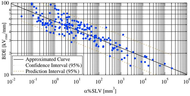
Fig. 5. Breakdown strength of LN<sub>2</sub> gap as a function of α%SLV.
