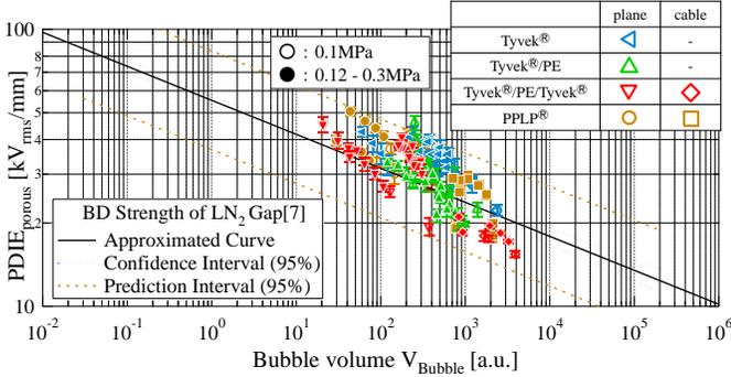
Fig. 6. Volume effect of PDIE for LN<sub>2</sub>/synthetic paper composite insulation system.
