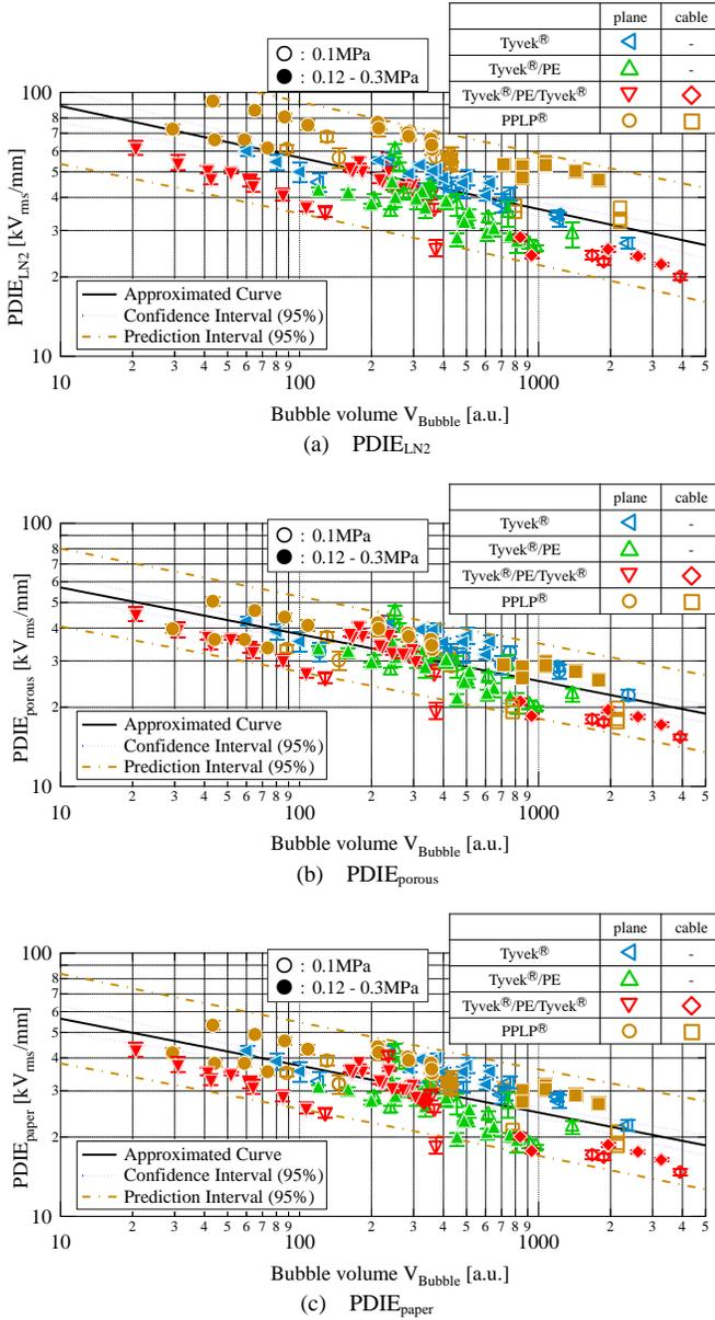
Fig. 3. PDIE strength of LN<sub>2</sub>/synthetic paper composite insulation system as a function of  $V_{\text{Bubble}}$ .
