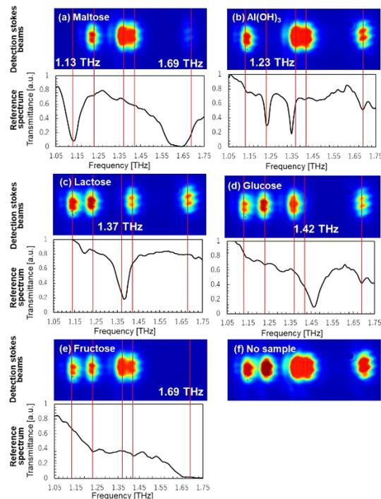
Fig. 5. Real-time measurement of reagents hidden in a cardboard box. (a–e) Detection Stokes beams with each sample inserted into the path of the THz-waves (upper figures) and the reference spectra of each sample obtained by an injection-seeded THz-wave parametric generator (lower figures). (f) Detection Stokes beams without samples. (see Visualization 1)
