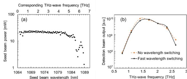
Fig. 2. (a) Tunability of an external cavity diode laser using a digital micromirror device; single-mode oscillation was confirmed. The upper axis shows the corresponding frequency (in THz) when the laser is used as a seed source for an injection-seeded THz-wave parametric generator. (b) Frequency tunability of the generator with (solid black line) and without (dashed orange line) fast wavelength-switching.
