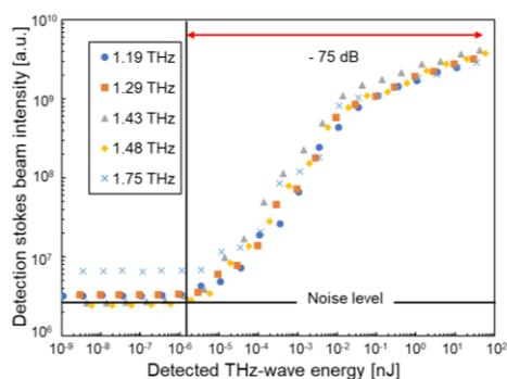
Fig. 4 Input-output characteristics during five-wavelength fast-switching. The dynamic range of this system was 75 dB because the detection Stokes beam could be detected down to an attenuation of 75 dB.
