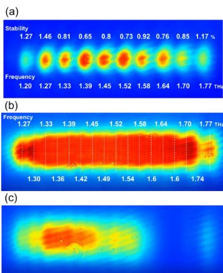
Fig. 3. Detection Stokes beams when (a) switching among 10 wavelengths (1.20–1.77 THz) and (b) switching among 17 wavelengths (1.27–1.77 THz). (c) Maltose was inserted into the THz-wave path while switching among the 17 wavelengths. The interference fringes in Fig. 3(b) and (c) were caused by the coverglass of the CMOS sensor of the NIR camera.
