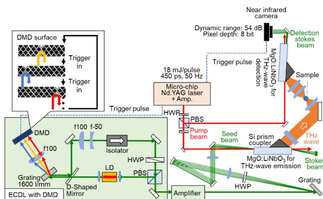
Fig. 1. Experimental setup of a rapidly wavelength-switchable injection-seeded THz parametric generator using an external cavity diode laser (ECDL) with a digital micromirror device (DMD).
