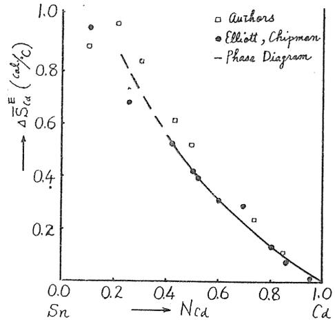
FIG. 5. Comparison between observed and calculated values for the excess molal entropy of cadmium.
