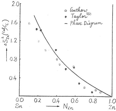
FIG. 4. Comparison between observed and calculated values for the excess molal entropy of zinc.
