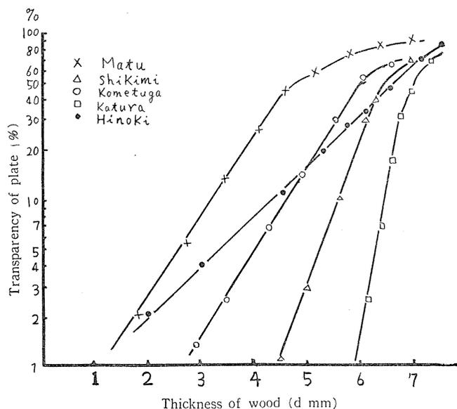
FIG. 4. Variation of plate transparency v.s. sample thickness.
