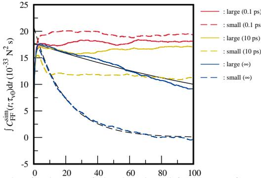
FIGURE 5 Integrating the time correlation function of the force on the methane molecule at  $\tau_{v0} = 0.1$  ps (red), 10 ps (yellow), and  $\infty$  (blue) in the large (solid line) and small (dashed line) systems. Eq. (19) of the large and small systems is shown by black solid and dashed lines.
