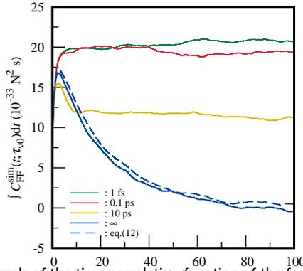
FIGURE 2 Running integrals of the time correlation function of the force on the methane molecule at  $\tau_{v0} = 1$  fs (green), 0.1 ps (red), 10 ps (yellow), and  $\infty$  (blue) in the smaller system. The curve calculated by the right-hand side of Eq. 14 is shown by the blue dashed line.
