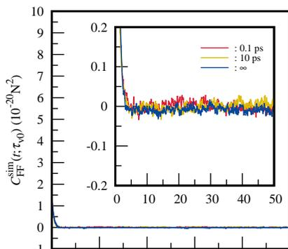
FIGURE 3 Time correlation function of the force on the methane molecule at  $\tau_{v0} = 0.1$  ps (red), 10 ps (yellow), and  $\infty$  (blue) in the large system. The inset shows a magnified view for  $0 \leq t \leq 50$  ps.
