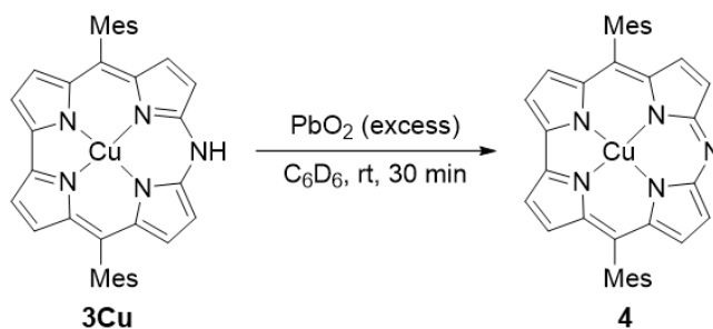
Scheme 2. The synthesis of type I copper azacorrrole 4 .
