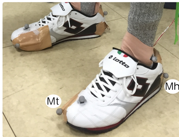
Fig.2.3 Shoe markers. Markers used to determine toe (Mt) and heel (Mh) distances to the ground in every step.
