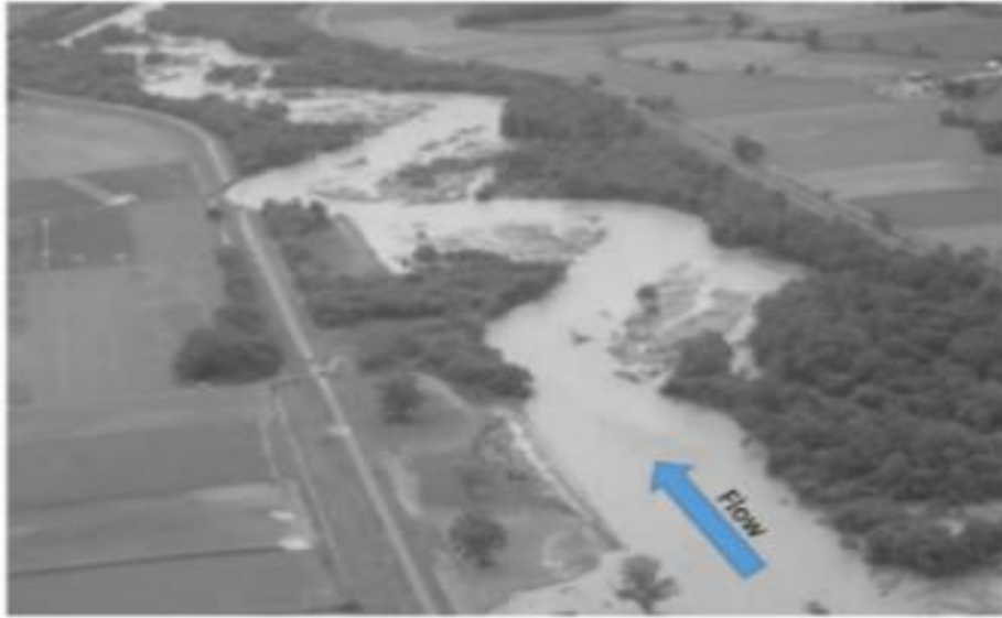
Figure 2.1 River meandering developed during the 2011 flood in the Otofuke River (Kawamura and Watanabe, 2015).
