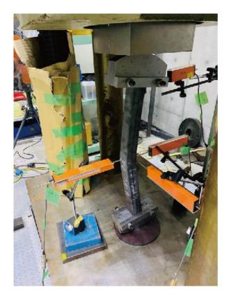
Figure 4.3.9 Deflection of the specimen after flexural buckling
