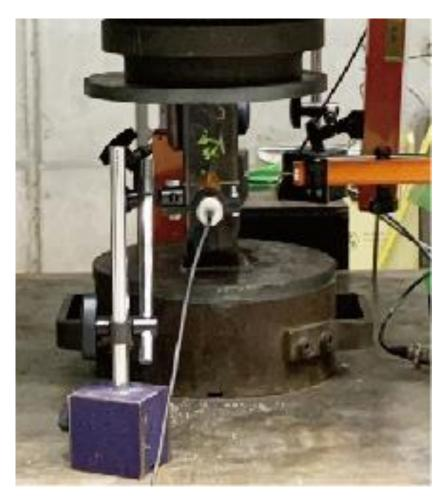
(a) Axially loaded stub-column test
