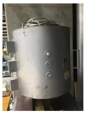
Figure 2.3.3 A cylindrical electric furnace
