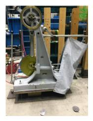
Figure 2.2.1 Charpy impact test machine
