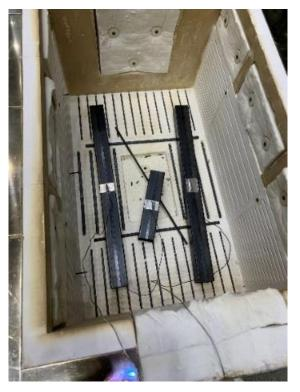
Figure 4.2.2. Specimens placed in an electric furnace
