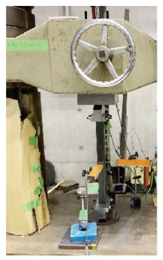
Figure 4.2.6. Axially loaded compressive test system
