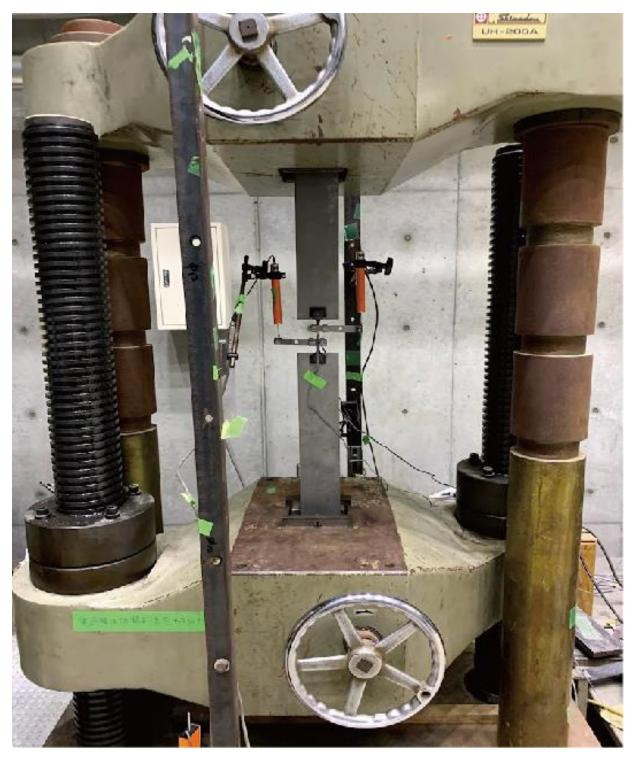
Figure 4.2.5 Coupon test
