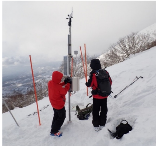
Fig. 3.2. Anemometer installed at Annupuri ((B) in Fig. 3.1).
