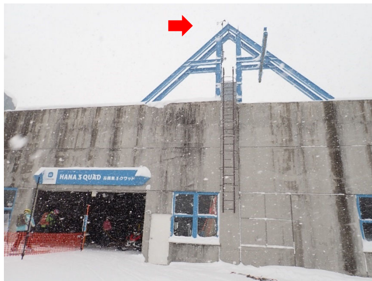
Fig. 3.3. Anemometer installed at Hanazono ((F) in Fig. 3.1).
