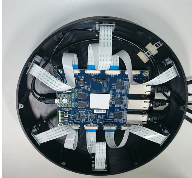
FIGURE 6.2: Picture of the FPGA board prototype.
