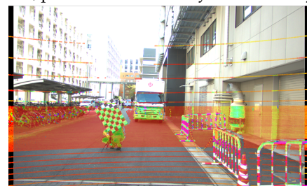
(H) Projection using \epsilon_C 's intrinsic parameters, point cloud colored by laser intensity.
