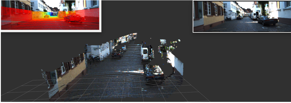
FIGURE 5.5: Result of the real time Image-Cloud fusion using a Velodyne HDL-64 and a wide-angle camera.
