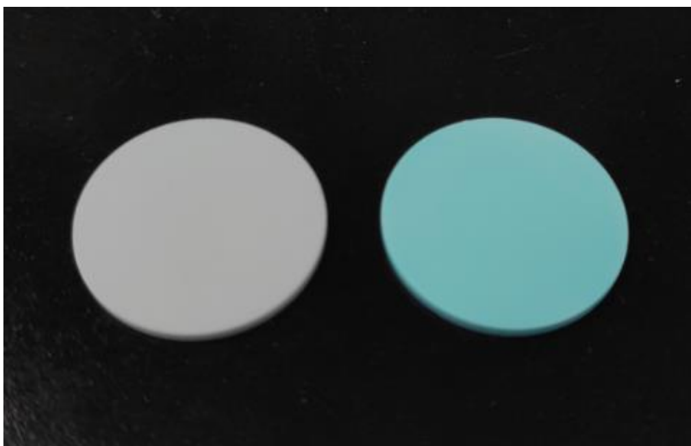
Figure 5-5. Optical images of the Al 2 O 3 support (left), Kgm-OPr seed layer after one cycle (right).
