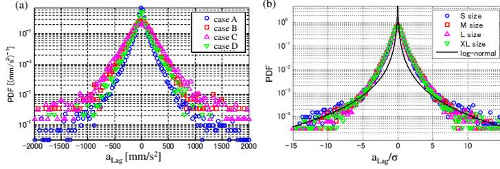
**Fig. 5** Lagrange acceleration in y-direction profile. (a) S size (b) case A. Solid line is log-normal distribution;  $P(a) = \frac{\exp(1.5S^2)}{4\sqrt{3}} \left[ 1 - \operatorname{erf} \left( \frac{\ln|a/\sqrt{3}| + 2S^2}{\sqrt{2}S} \right) \right]$  with  $S = 1.5$ . (Color figure online).
