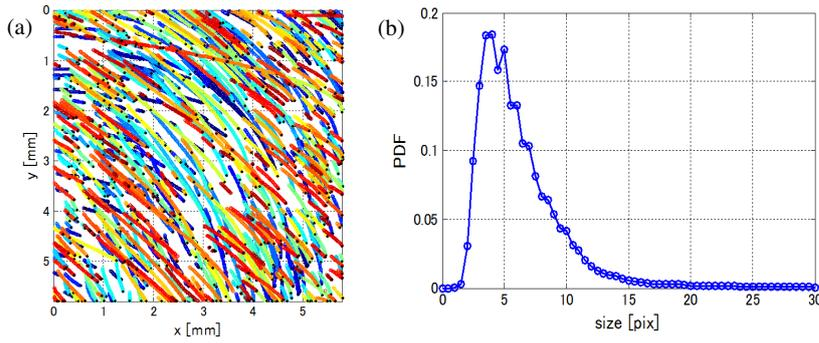
**Fig. 2** (a) particle trajectory, (b) particle size distribution (Color figure online).
