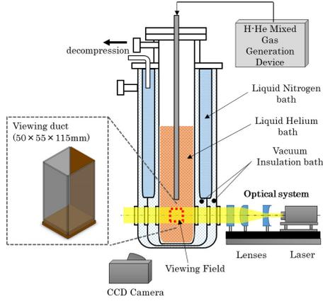
**Fig. 1** Schematic view of experimental apparatus (Color figure online).
