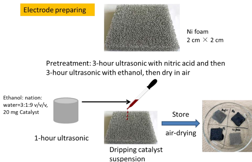
Fig. 5- 2 Diagram of preparing process for catalytic electrodes.
