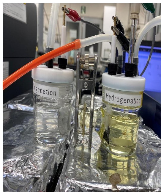
Fig.4. 3 Schematic (left) and photograph (right) of electrochemical reactor
