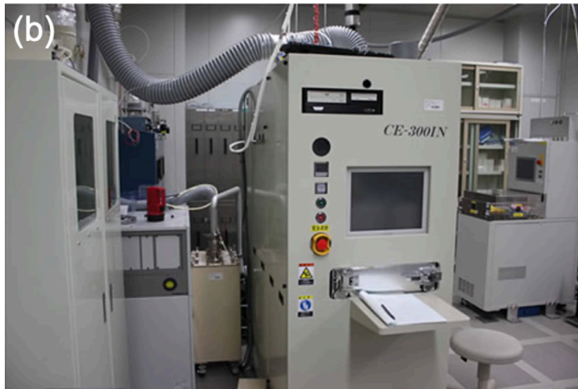
Figure 2.5 (b): ICP-RIE system (CE-300I).
