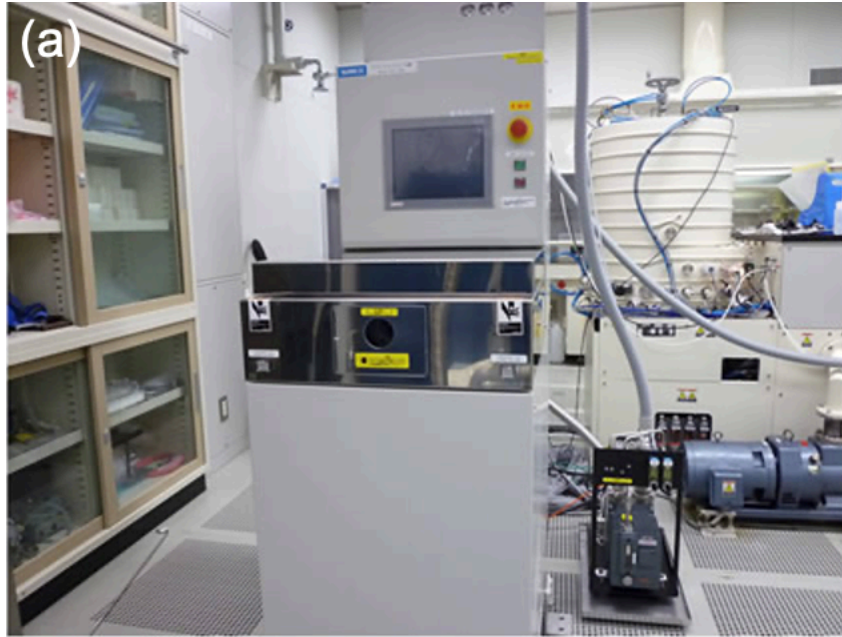
Figure 2.5 (a): Parallel plate reactive ion etching system (RIE-10NR).
