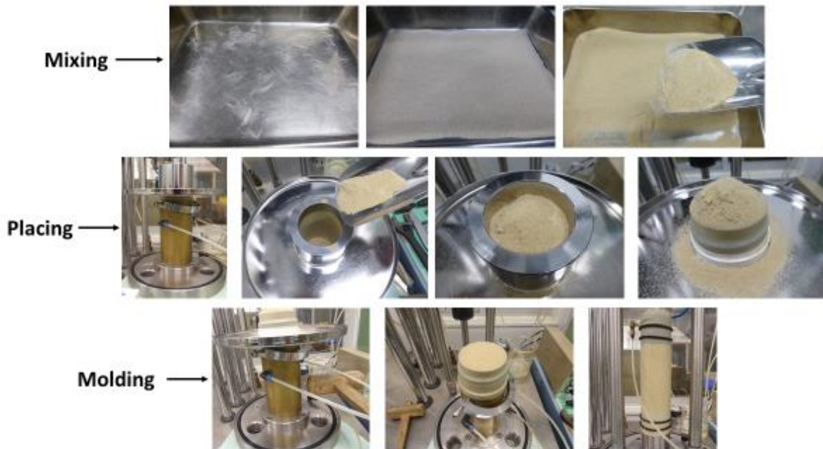
Fig. 3.8 Sample preparation of fiber-reinforced sand (example of 0.4% fiber content)
