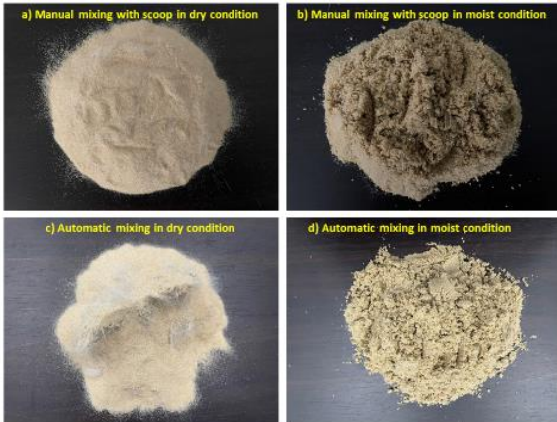
Fig. 3.9 Sand – fiber admixture after the mixing process performed in 4 different methods
