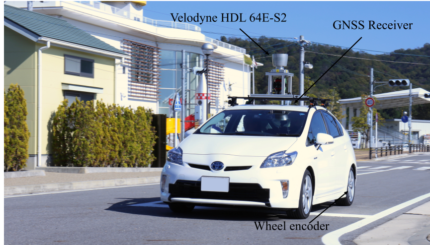
Figure 3-5: Experimental vehicle equipped with 3D LiDAR , GNSS receiver and wheel encoder.
