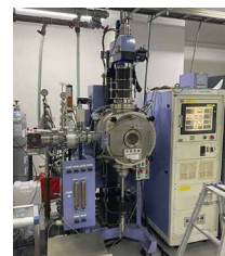
高周波加熱型SiC結晶成長炉 (小型) High frequency induction heating furnace for SiC crystal growth (large type)
