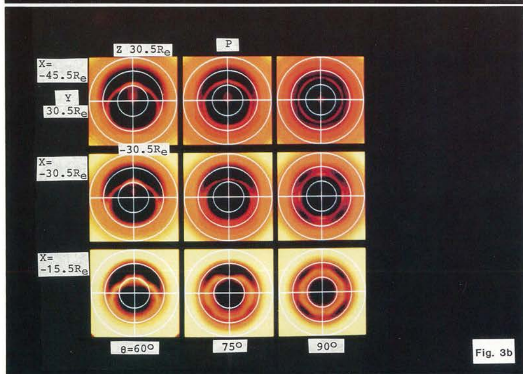
Fig. 3a. and 3b. Structure of the plasma sheet in the tail cross section depending on the dipole tilt angles, \theta = 0^\circ \sim 90^\circ , where the plasma pressure is depicted by color code.
