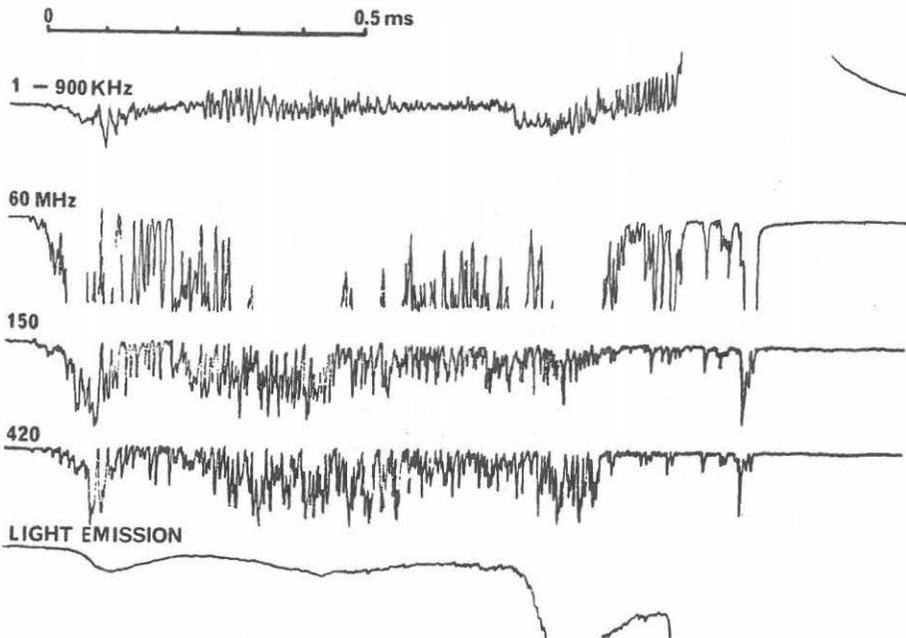
Fig. 3. Fast display of the second ground stroke of the same flash as shown in Fig. 1. Much more intense radiation accompanies dart leader process rather than return stroke.
