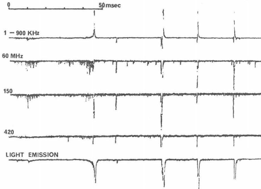
Fig. 1. Slow display of electric field change, radiations at three frequencies and light emission. The figure includes from the stepped leader process followed by the first return stroke through the fourth return stroke.
