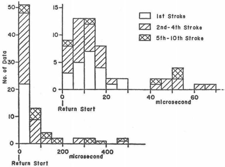
Fig. 5. Distribution of start-time of return type radiation at 60 MHz (Types 2 and 3). Upper-right figure shows the detailed distribution of start-time smaller than 70  $\mu$ sec, where most of data are included.
