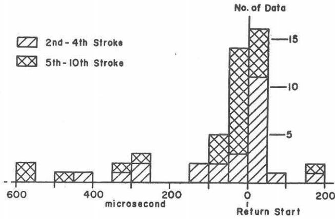
Fig. 4. Distribution of end-time of dart leader type radiation at 60 MHz (Types 1 and 3). Left-hand and right-hand sides of 0 respectively mean the time before and after the return stroke starts from the ground.
