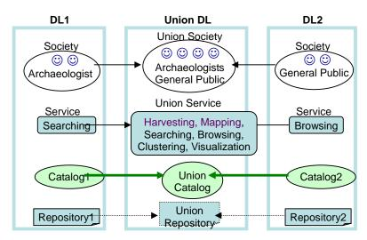
Fig.5 Architecture of a union DL
