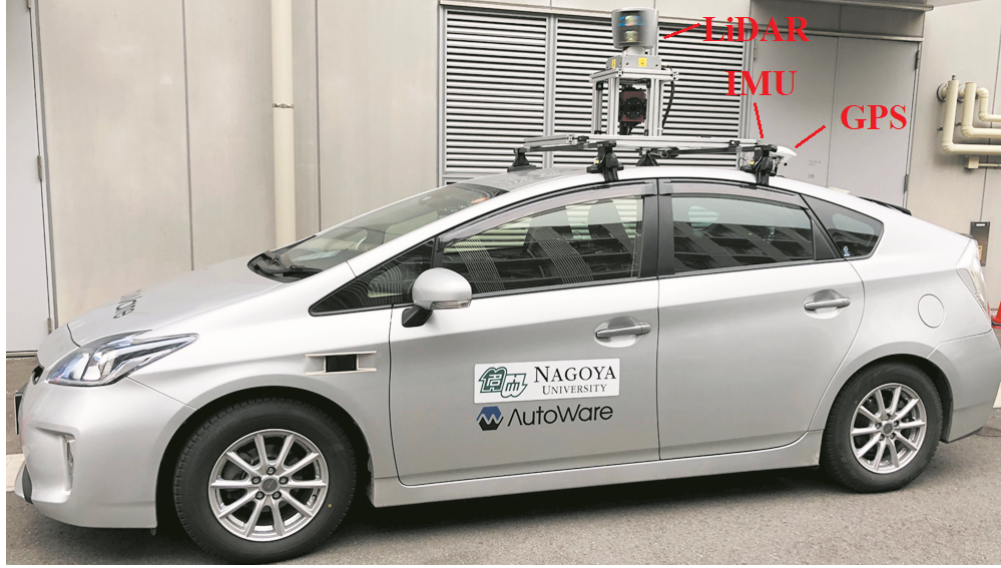
Figure 3.2: Involved sensors in this dissertation: the LiDAR: Velodyne HDL-64ES3; the GPS: Trimble NetR9; the IMU: Xsens MTi-300.
