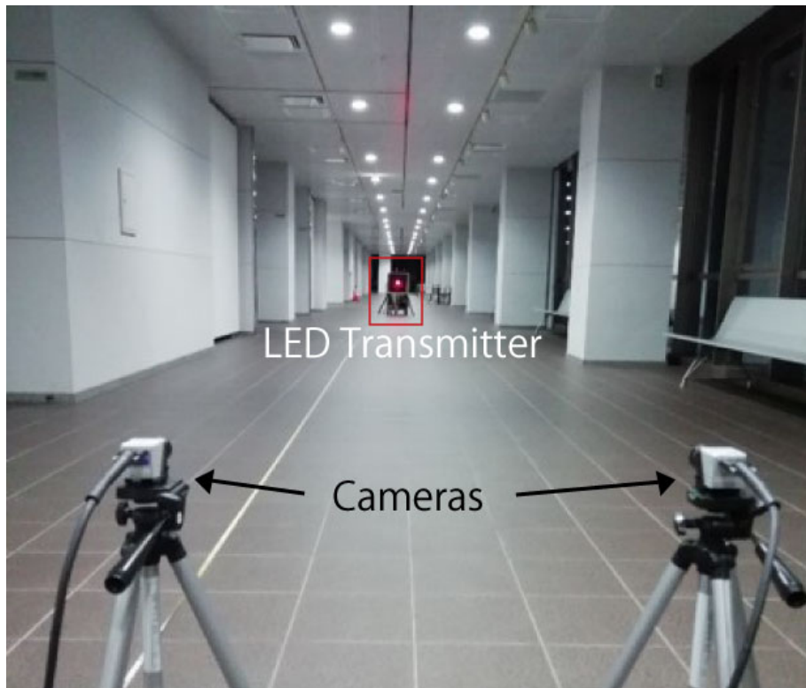
Figure 3.6: Photograph showcasing the experimental setup. The LED transmitter is highlighted within a red rectangle.
