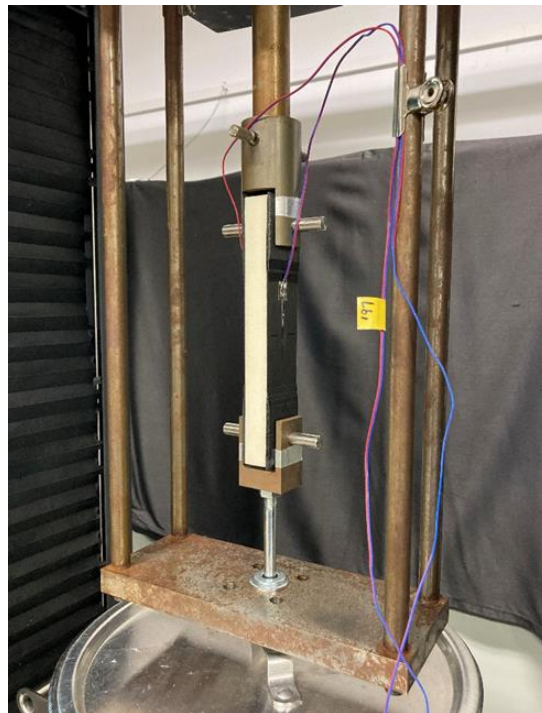
Fig.3.5-3 CFRP Sandwich tensile test setup
