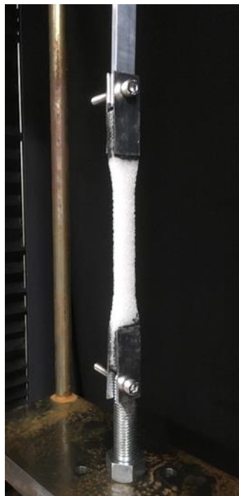
Fig.2.2-9 Setup of foam tensile test (RT)
