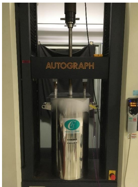
Fig.2.3-2 Overview of cryogenic load test
