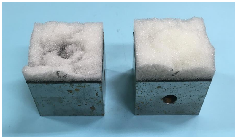
Fig.2.3-12 Failure pattern of flatwise tension specimen (CT1)
