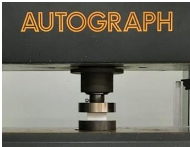
Fig.2.2-4 Overview of foam compression test (RT)
