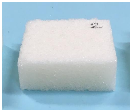
Fig.2.3-4 Test specimens after compression test (CT)
