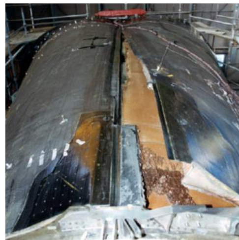
Fig.1.1-5 Honeycomb sandwich failure at X-33 cryogenic composite tank development [14]
