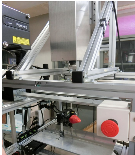
Figure 4-1. Strawberry Rotation line scan measurement system using NIR-HSI system and laser displacement meter
