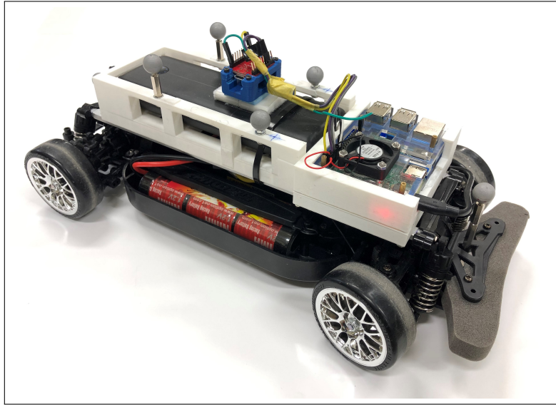
Fig. 3.8 RC car with attached computer and markers for localization
