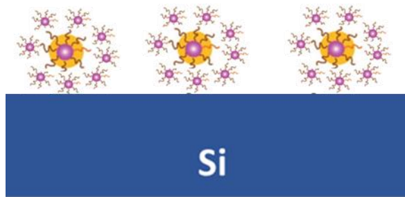
Fig. A2.4. Schematic diagram of core-satellite structure by Au-Ag core-shell nanoparticles on Si surface.
