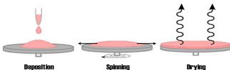
Figure 2.4. Schematic diagram of spin coating process.
