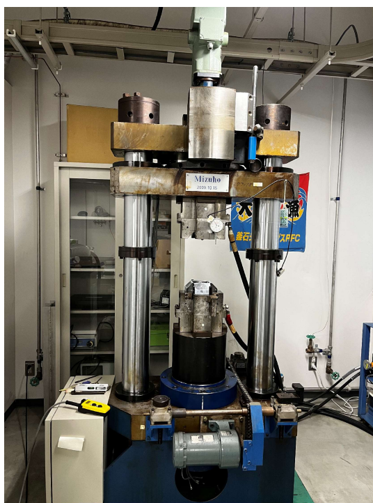
Figure 2-1 250-ton DIA-type cubic multi-anvil large volume press.
