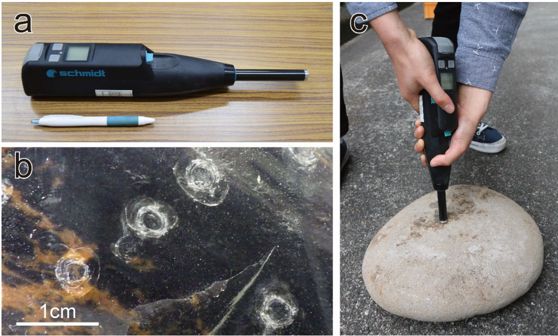
Fig. 4.1. a) Schmidt Hammer used in this study. b) Punch marks on obsidian, left by Schmidt Hammer after measurement. c) Scene during the use of Schmidt Hammer on a grinding quern made of andesite.
