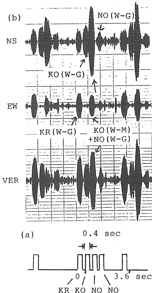
Fig. 2 (a) Transmission format of the 14.881 kHz signals.
