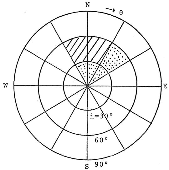
Fig. 7 Distribution of the arrival directions of the 14.881 kHz whistler-mode waves. The distribution is depicted by occurrence rates in 36 segments divided by every 30° in azimuthal and incident angles.
