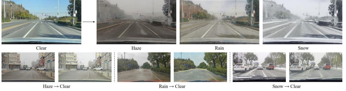
Figure 3.8: MWCG translates clear images into rainy, snowy, or foggy images using three different generators, creating a set of images representing different weather conditions (top row). In contrast, only one generator is needed to translate all three types of adverse weather images into clear ones (bottom row).
