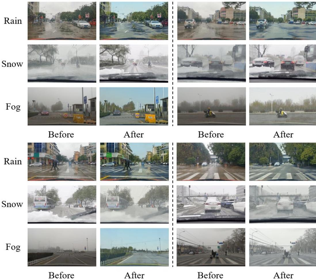
Figure 3.11: Weather removal results for the RDSBW dataset, showing examples of MWCG’s translation of adverse weather images into clear weather images. While MWCG was unable to recover objects and buildings hidden behind dense fog, it did not randomly insert fake objects.
