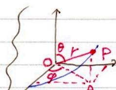
$$\begin{aligned} \overline{OP} &= \sqrt{\overline{OA}^2 + \overline{PA}^2} \\ &= \sqrt{l^2 + (ut)^2} \\ \theta(t) &= \arccos \left( \frac{ut}{\sqrt{l^2 + (ut)^2}} \right) \\ \varphi(t) &= \omega t \end{aligned}$$
