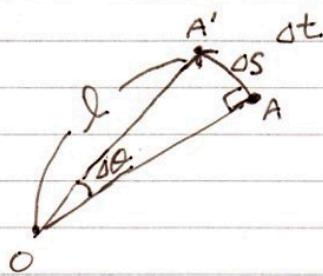
$$\text{速さ } v(t) \underset{\Delta t \rightarrow 0}{=} \lim_{\Delta t \rightarrow 0} \frac{\Delta s}{\Delta t} \approx \lim_{\Delta t \rightarrow 0} \frac{l \sin(\theta)}{\Delta t}$$
