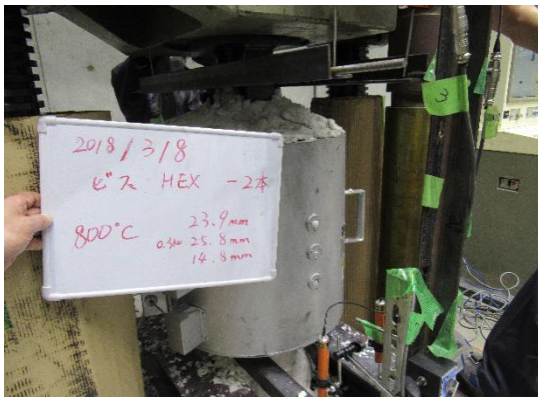
Fig 2.7 Testing jig for shear tests and test systems
