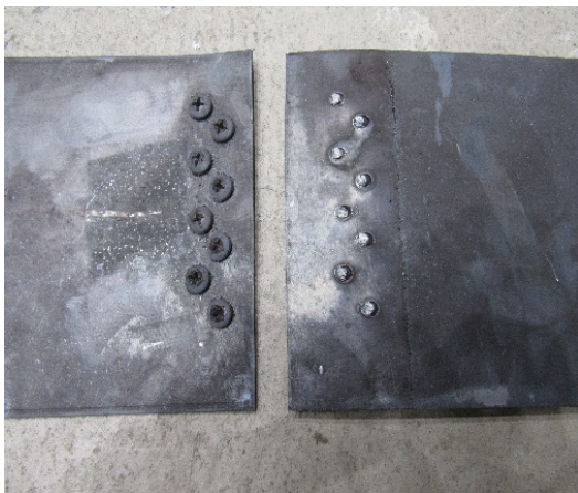
600°C Screw shear failure (Type4)
