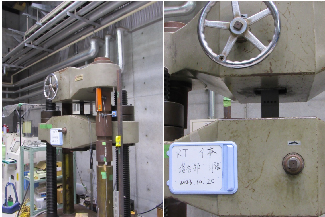
Fig 5.4 Test set-up of screwed connection specimens
