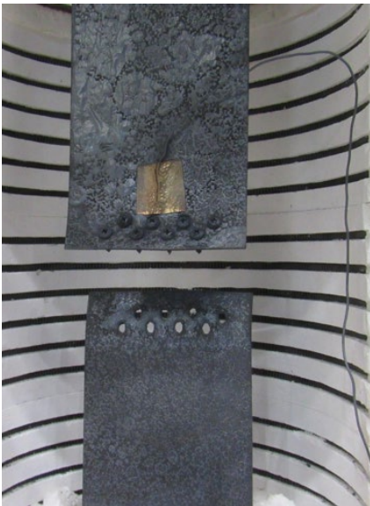
800°C Sheet bearing failure (Type2)
