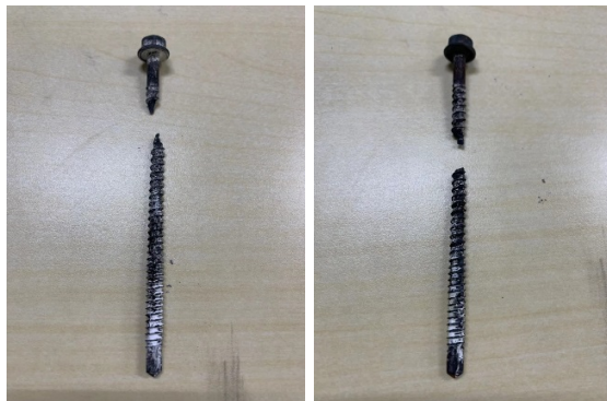
Fig 2.4 Photographs of ASUS after tensile test
