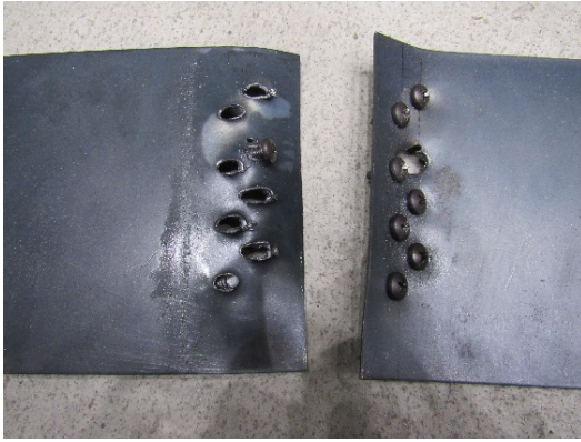
RT Sheet bearing failure (Type2)
