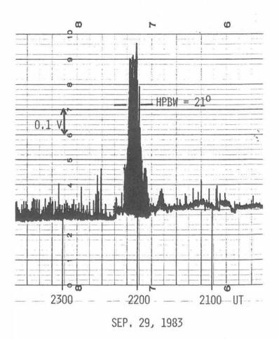
Fig. 3. Recording of the beacon signal of the RS-7 satellite at 29.340 MHz for the Orbit No. 7858. Output level is proportional to the received electric field strength.
