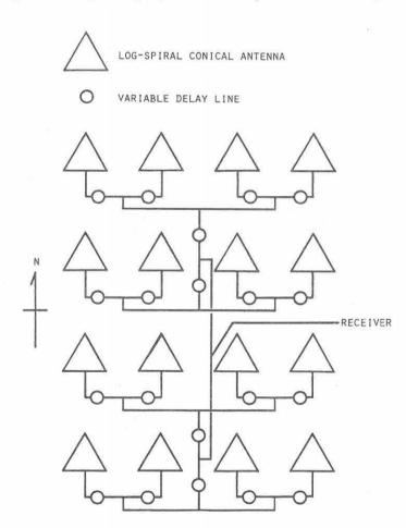
Fig. 2. A block diagram of the receiving system.
