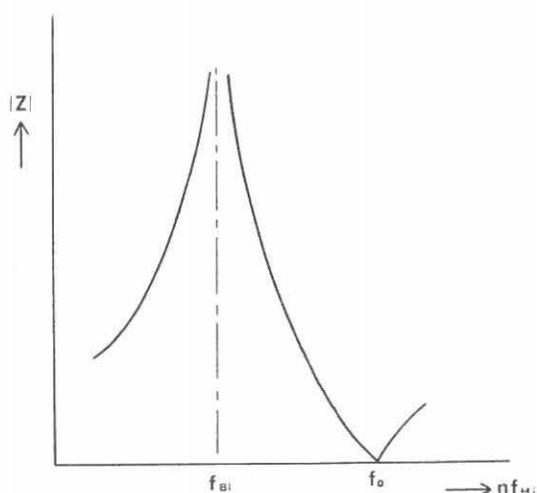
Fig. 3. The variation of antenna impedance.
