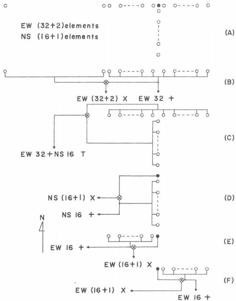
Fig. 1. Various modes of operation of 8-cm radio interferometer system.
