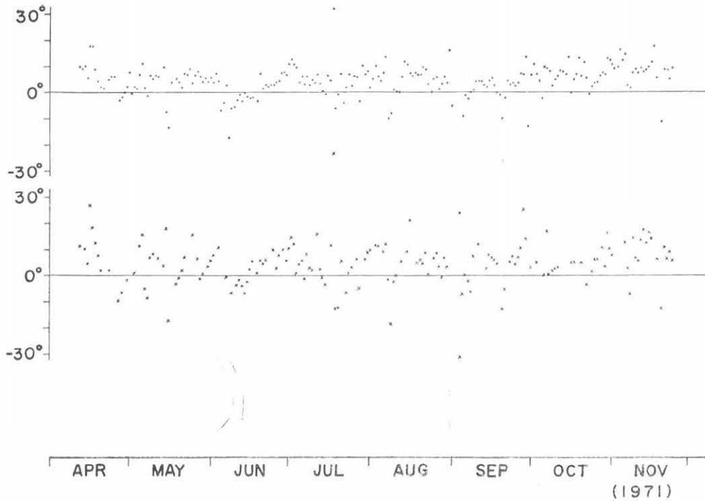
Fig. 2. Daily variations of the phase error between the adjacent two antennas.
