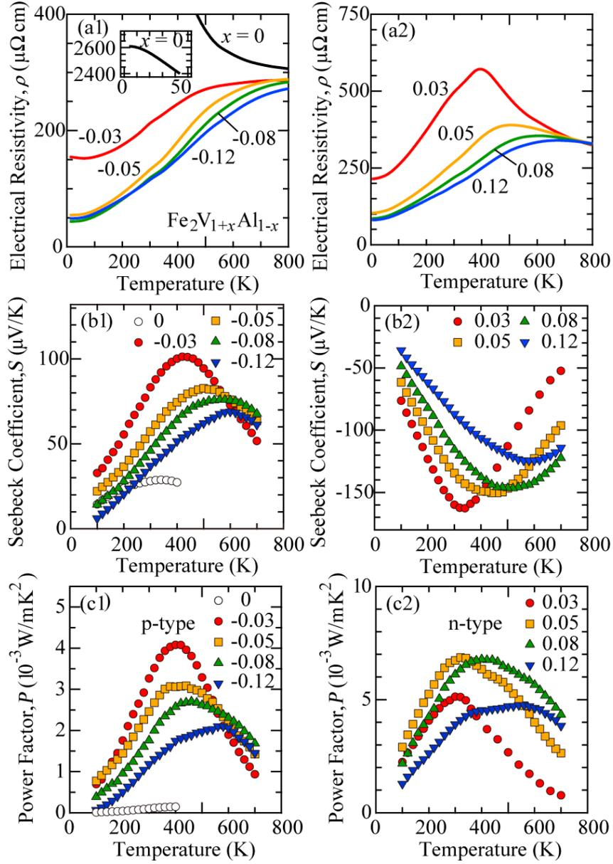
**Figure 2.** Temperature dependence of the electrical resistivity,  $\rho$ , Seebeck coefficient,  $S$ , and thermoelectric power factor,  $P$ , in  $\text{Fe}_2\text{V}_{1+x}\text{Al}_{1-x}$  alloys with compositions of  $-0.12 \leq x \leq 0$  (a1, b1, c1) and  $0 < x \leq 0.12$  (a2, b2, c2). The inset shows the  $\rho$  of  $\text{Fe}_2\text{VAl}$  in the low-temperature region.
