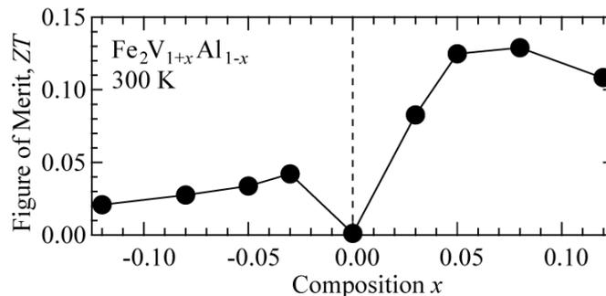
**Figure 4.** Figure of merit,  $ZT$ , in  $\text{Fe}_2\text{V}_{1+x}\text{Al}_{1-x}$  alloys with compositions of  $-0.12 \leq x \leq 0.12$  at 300 K.
