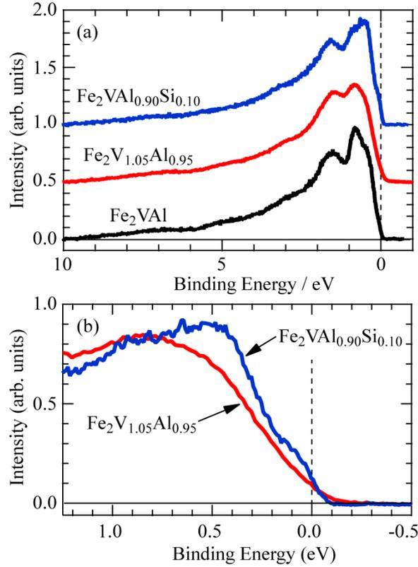
**Figure 6.** The valence band photoemission spectra of wide energy range (a) and near the Fermi level (b) of Fe<sub>2</sub>VAl, Fe<sub>2</sub>V<sub>1.05</sub>Al<sub>0.95</sub> and Fe<sub>2</sub>VAl<sub>0.90</sub>Si<sub>0.10</sub> recorded at  $h\nu = 900$  eV.
