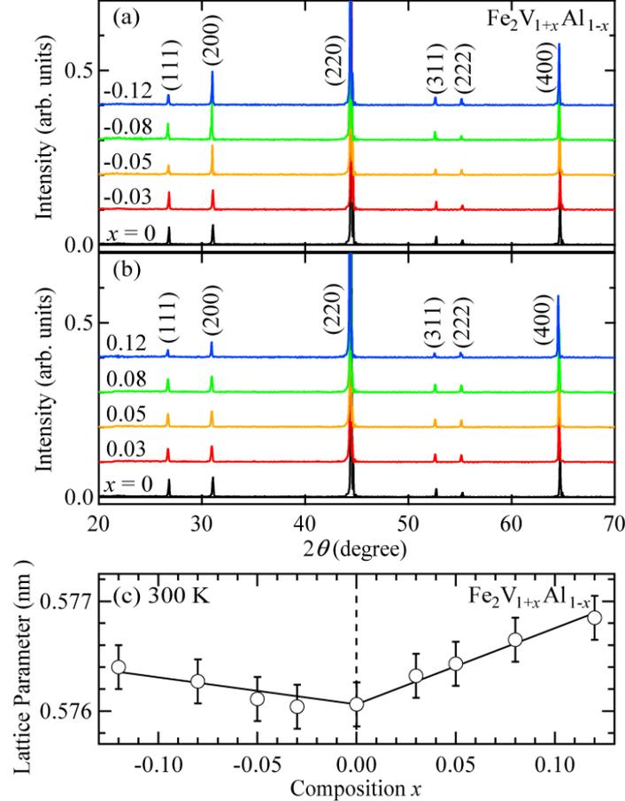
**Figure 1.** XRD patterns of powdered  $\text{Fe}_2\text{V}_{1+x}\text{Al}_{1-x}$  alloys with compositions of  $-0.12 \leq x \leq 0$  (a) and  $0 \leq x \leq 0.12$  (b). (c) Lattice parameters of  $\text{Fe}_2\text{V}_{1+x}\text{Al}_{1-x}$  with compositions of  $-0.12 \leq x \leq 0.12$  determined from the XRD patterns (open circles). The lines show the fitting results of these lattice parameters using a linear function.
