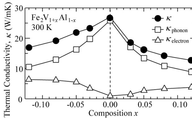
**Figure 3.** Thermal conductivity (filled circles),  $\kappa$ , of  $\text{Fe}_2\text{V}_{1+x}\text{Al}_{1-x}$  alloys with compositions of  $-0.12 \leq x \leq 0.12$  at 300 K. The open squares and triangles indicate the phonon and electron component of the  $\kappa$  determined by the Wiedemann-Franz law, respectively.
