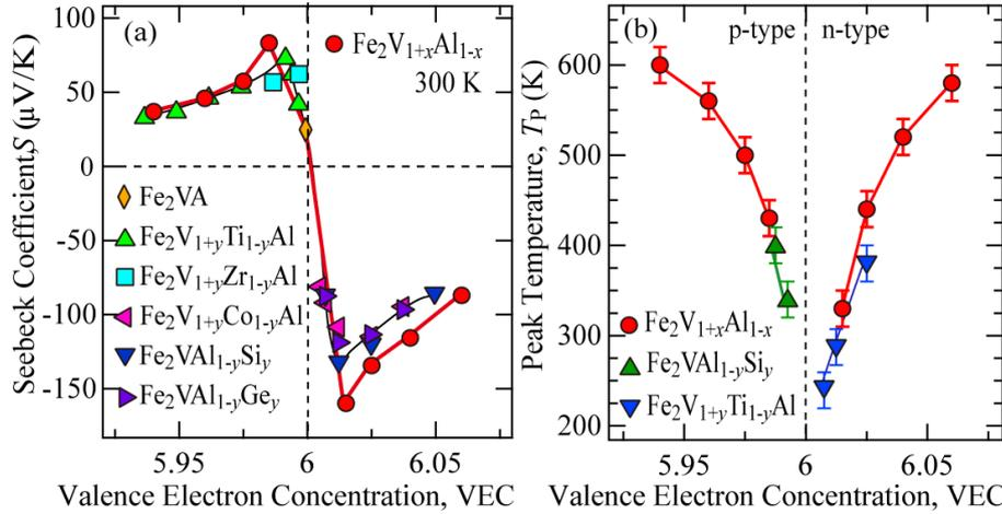
**Figure 5.** Valence electron concentration (VEC) dependence of the experimental Seebeck coefficient,  $S$ , at 300 K (a) and peak temperature,  $T_p$ , determined by  $S$  (b) in typical Fe-based Heusler and  $\text{Fe}_2\text{V}_{1+x}\text{Al}_{1-x}$  alloys.
