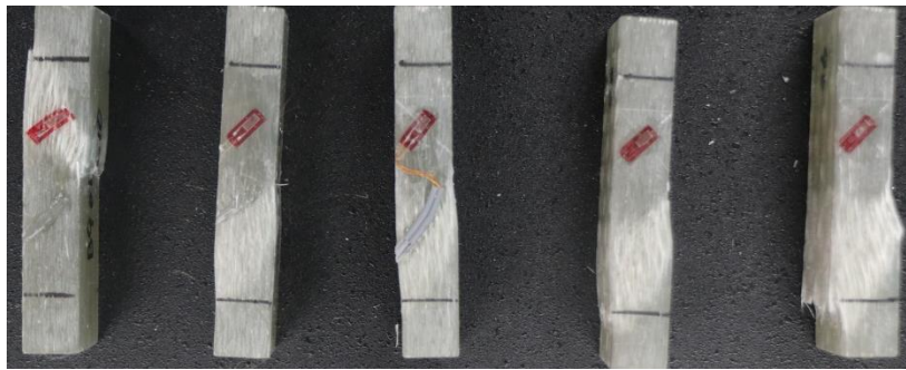
Figure 4.14: Failure mode of short beam test specimen
