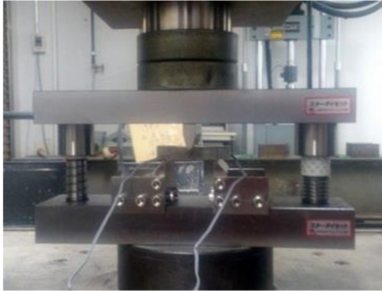
Figure 4.13: Setup of short beam test specimen
