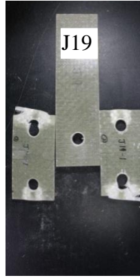
(b) Shear failure
