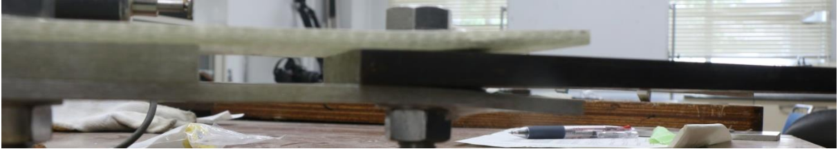
Figure 4.28: Bending effect in cover plate
