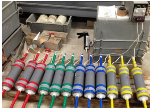
Figure 2.13 Preparation of corroded rebar specimens by electric corrosion method
