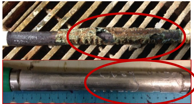
Figure 2.18 Experimental observation (corrosion products adhered to rebar surface)
