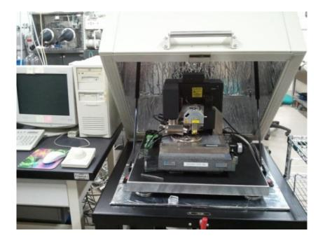
Figure 2.7 Atomic force microscope (Dimension 3199 SPM, Veeco).
