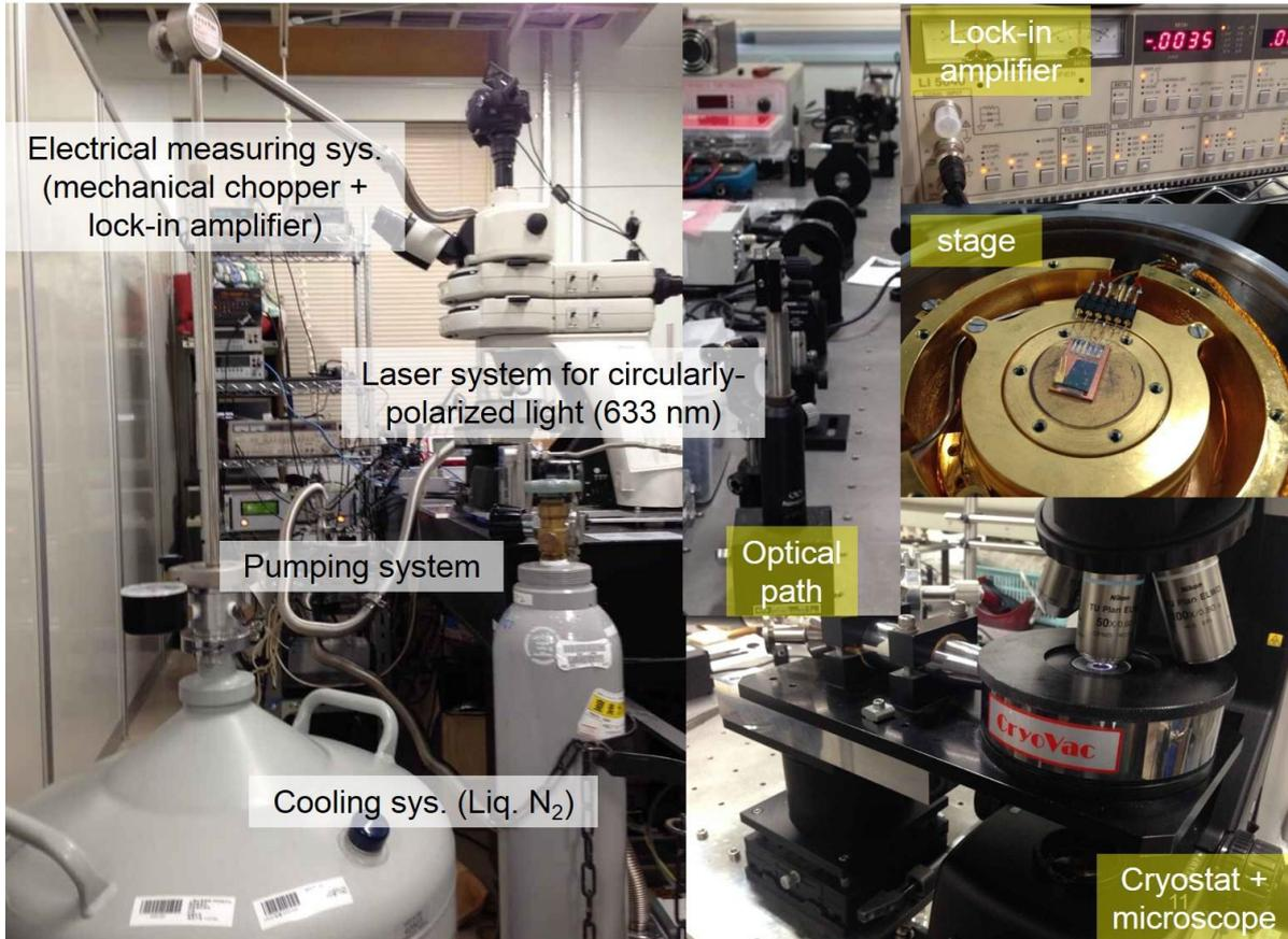
Figure 6. A set of photos displaying the instrumental set-up used in the measurement of valley transport.
