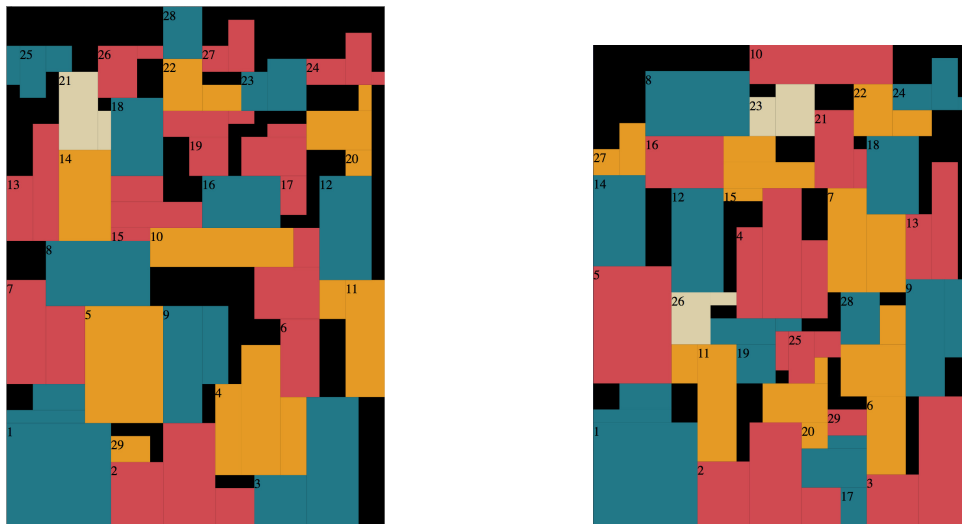
Figure 6.1: An example when the best-fit algorithm performs better (left: the bottom-left algorithm, right: the best-fit algorithm)
