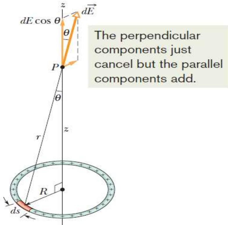
**Fig. 22-10** A ring of uniform positive charge. A differential element of charge occupies a length  $ds$  (greatly exaggerated for clarity). This element sets up an electric field  $d\vec{E}$  at point  $P$ . The component of  $d\vec{E}$  along the central axis of the ring is  $dE \cos \theta$ .
