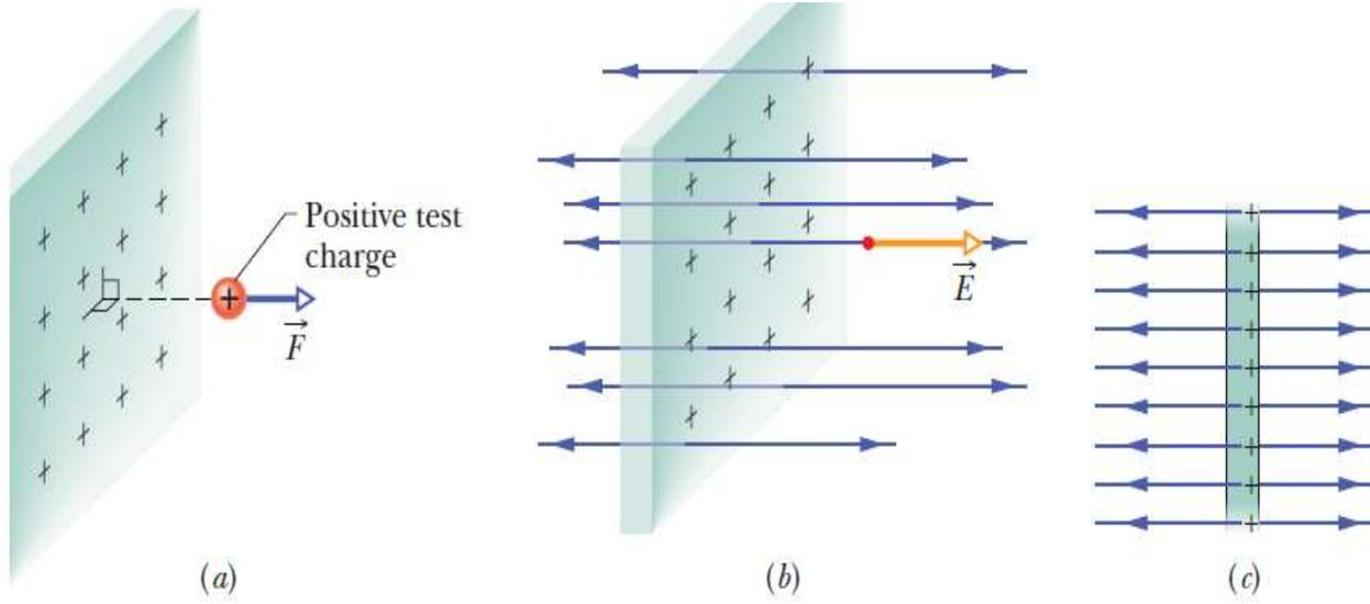
**Fig. 22-3** (a) The electrostatic force  $\vec{F}$  on a positive test charge near a very large, nonconducting sheet with uniformly distributed positive charge on one side. (b) The electric field vector  $\vec{E}$  at the location of the test charge, and the electric field lines in the space near the sheet. The field lines extend *away from* the positively charged sheet. (c) Side view of (b).
