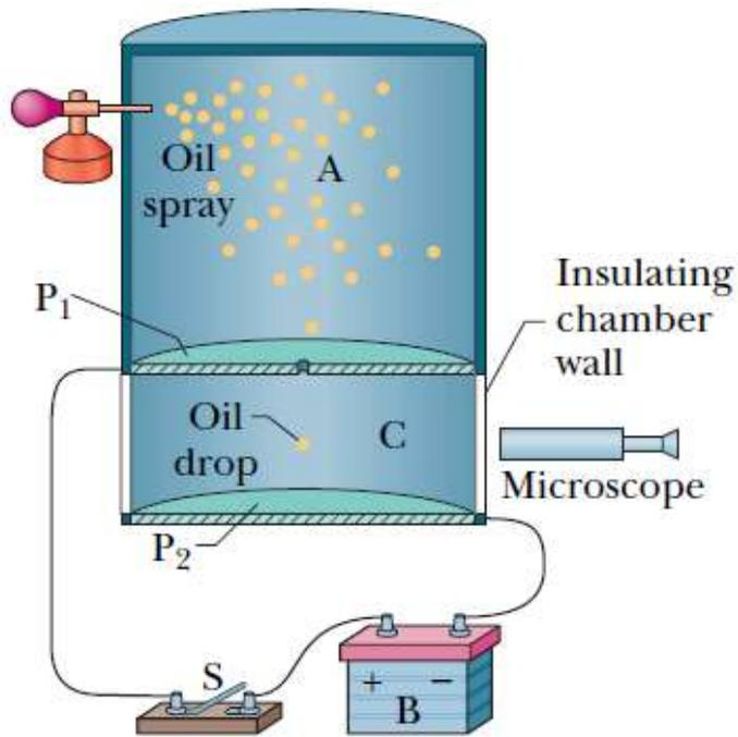
**Fig. 22-14** The Millikan oil-drop apparatus for measuring the elementary charge  $e$ . When a charged oil drop drifted into chamber C through the hole in plate P<sub>1</sub>, its motion could be controlled by closing and opening switch S and thereby setting up or eliminating an electric field in chamber C. The microscope was used to view the drop, to permit timing of its motion.
