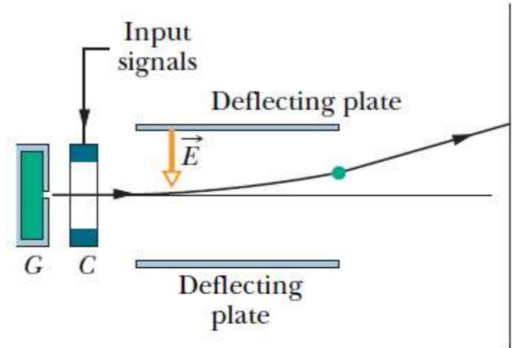
**Fig. 22-15** Ink-jet printer. Drops shot from generator  $G$  receive a charge in charging unit  $C$ . An input signal from a computer controls the charge and thus the effect of field  $\vec{E}$  where the drop lands on the paper.
