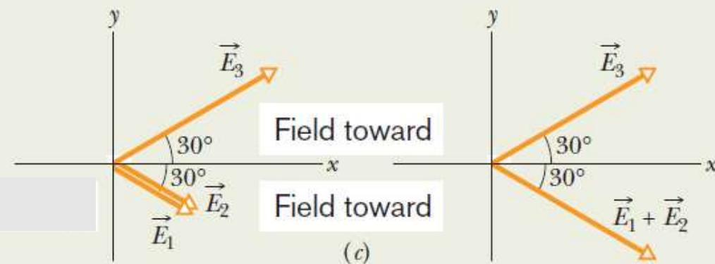
**Fig. 22-7** (a) Three particles with charges  $q_1$ ,  $q_2$ , and  $q_3$  are at the same distance  $d$  from the origin. (b) The electric field vectors  $\vec{E}_1$ ,  $\vec{E}_2$ , and  $\vec{E}_3$ , at the origin due to the three particles. (c) The electric field vector  $\vec{E}_3$  and the vector sum  $\vec{E}_1 + \vec{E}_2$  at the origin.
