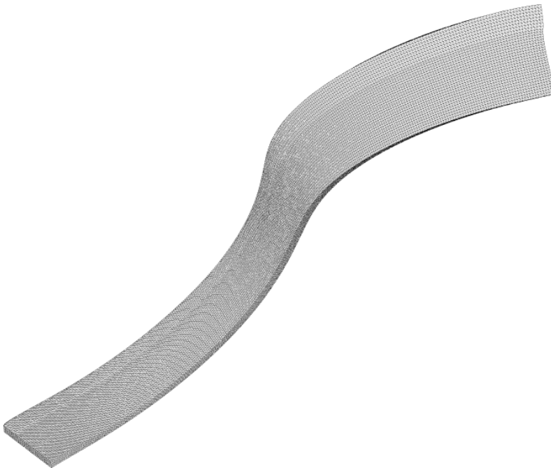
Figure 3.9: The 2nd Mode from nonlinear growth deformations of plate model with initial imperfections ( \lambda = 45.59 )
