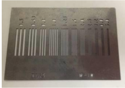
Fig. 3-6 Tungsten resolution chart used for spatial resolution evaluation
